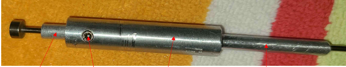
Tensioner Grub Screw Tensioner Housing Pick guide / Pick Set Piece
